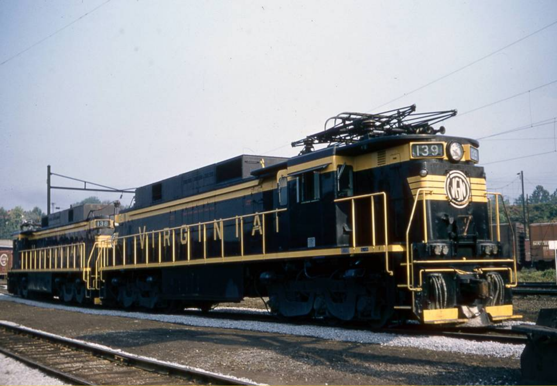
Brand new rectifier electric locomotives just delivered from GE. The older electrics had already been retired. Roanoke, VA August 31, 1957.
